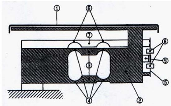
**Fig.2 Electronic Balance Sensor type vibrating string**
